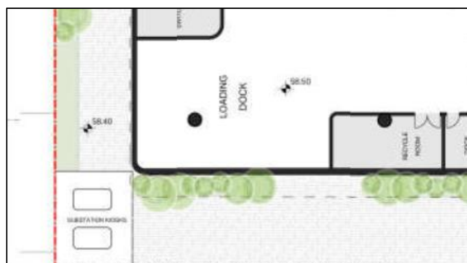
Figure 16. Extract of ground floor plan showing the proposed location of the substation kiosks, with the through-site link (source: 3XN)
